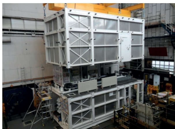
Waste tipping and package loading modules at works testing site.
