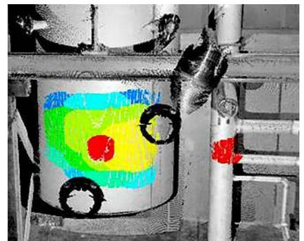
Scanned Image of Phase 2 Demonstration Cell with radiological overlay.
