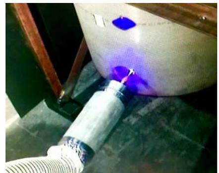
Phase 2 Inactive Demonstration laser cutting operations.
