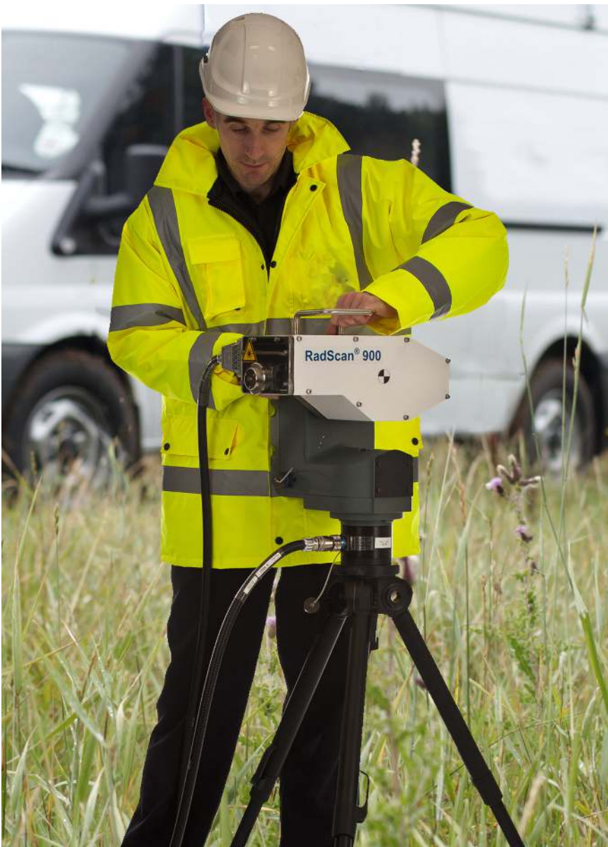
Setting up the RadScan® 900 detector head and tripod prior to deployment.
