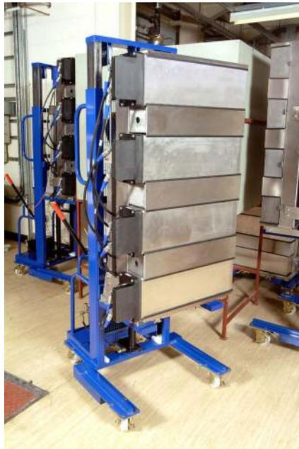
DISPIM® detector assembly comprising 4 modules.
