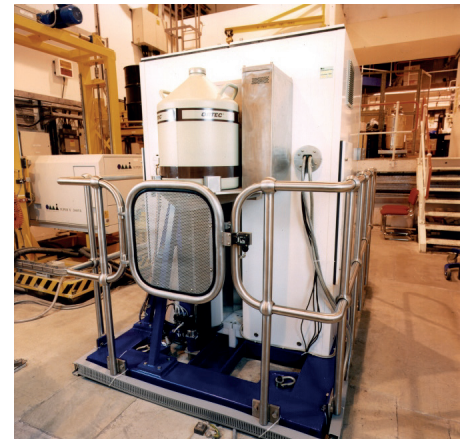
The TRU-D® Drum monitor being tested and set up at Cavendish Nuclear's facility prior to shipping to the client
