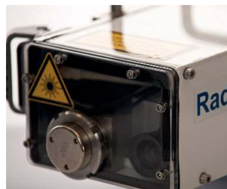
RadScan® 900 Detector Head showing collimator (bottom left) video camera (bottom right) and laser rangefinder
