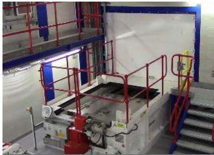
The newly designed bespoke equipment for removing the door/seal from the SP/2055 Package.
