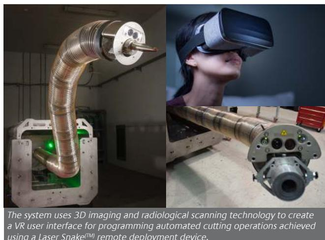
The system uses 3D imaging and radiological scanning technology to create a VR user interface for programming automated cutting operations achieved using a Laser Snake™ remote deployment device.
